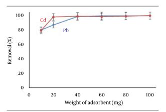
Figure 5. Effect of Magnetic Zero-Valent Iron Nanoparticles Amount for Quantitative Removal of Pb(II) and Cd(II) Using Magnetic Zero-Valent Iron Nanoparticles at 25°C
