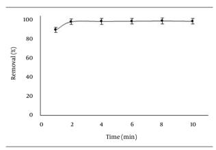
Figure 4. Effect of Stirring Time on the Removal of Pb(II) and Cd(II) Using Magnetic Zero-Valent Iron Nanoparticles at  $25^{\circ}$ C
