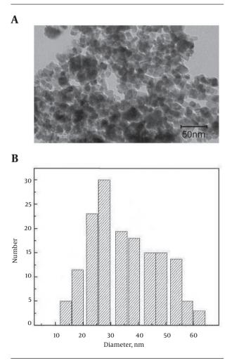
Figure 1. TEM Image (A) and Graph of Size Distribution (B) of the Synthesized Magnetic Zero-Valent Iron Nanoparticles
