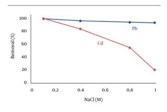
Figure 7. Effect of NaCl on Removal Efficiency of Pb and Cd Ions in the Solution
