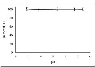
Figure 3. The Effect of pH on Removal of Pb(II) and Cd(II) Using Magnetic Zero-Valent Iron Nanoparticles at  $25\,^\circ\text{C}$
