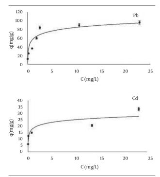
Figure 6. Plot of q Versus C at  $25^{\circ}$ C and pH = 9.0 With Langmuir Model Fit of the Data for Pb(II) and Cd(II)
