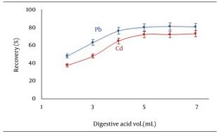
**Figure 8.** Effect of Volume of Acidic Digesting Solution (4:1 HNO<sub>3</sub>:H<sub>2</sub>SO<sub>4</sub>) on Recovery of Pb and Cd Ions Using Zero-Valent Iron Nanoparticles as a Solid Phase Extractor
